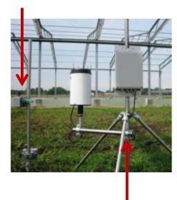
Measuring stations (1x per Block: rain und radiation measurement)
