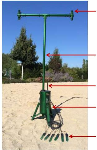
Optical sensors: photosynthetically active radiation (PAR) and 4 wavelength specific sensors (net balance)
